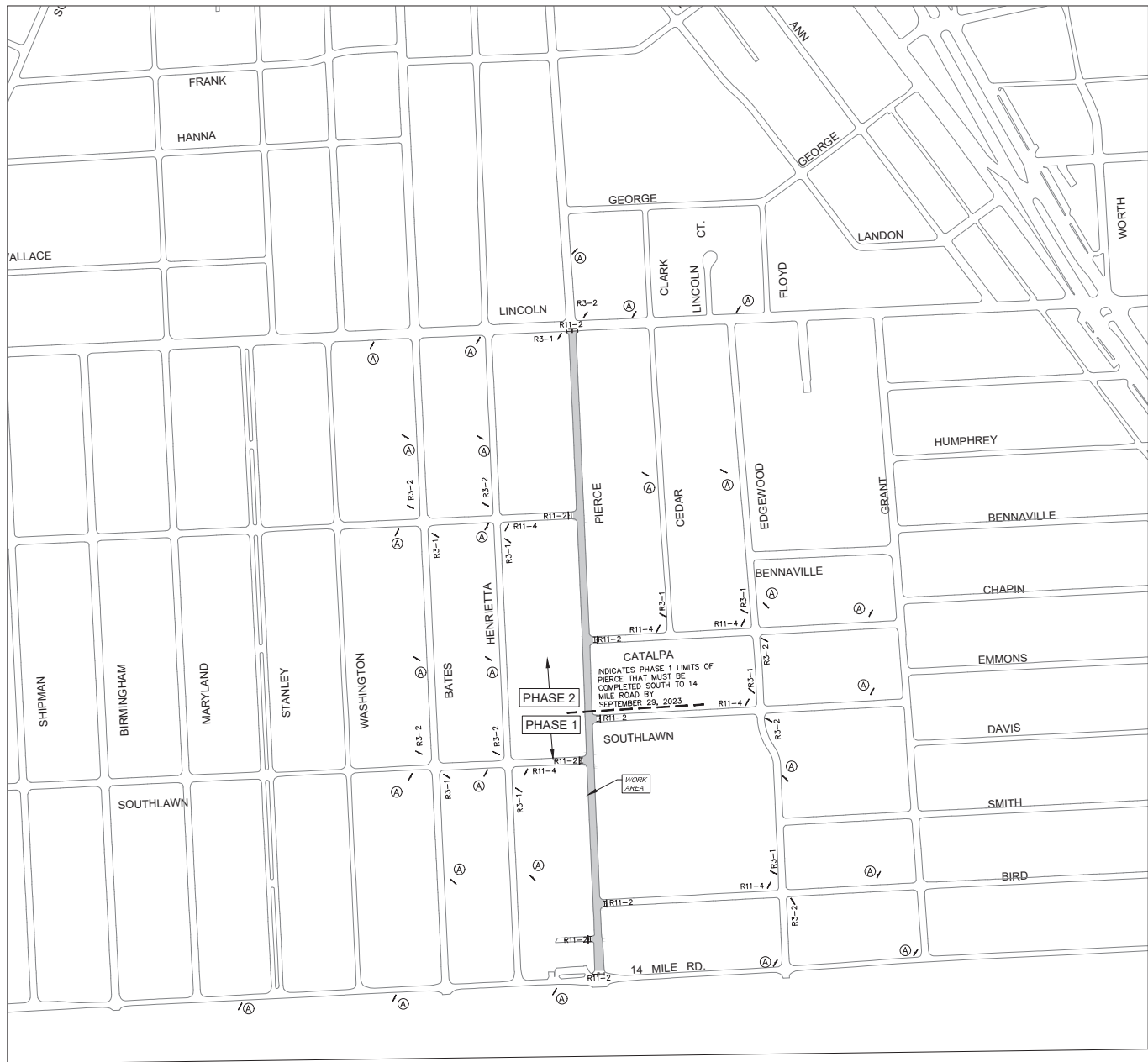
ADVANCED WARNING SIGNAGE & DETOUR PLAN: PIERCE ST.
